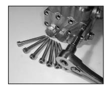
5) Use a 8mm allen wrench to remove the 8 socket head cap screws (34). Carefully slide the valve casing (26) out over the plungers. Remove the weep return rings (25).
